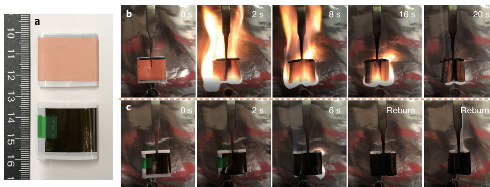
Fig. 5 | Fire retardancy test on full pouch cells assembled using Al/Cu CC and PI-TPP-Al/PI-TPP-Cu CC pairs. a , Photos of the assembled Cu/Gr||LCO/Al (top) and PI-TPP-Cu/Gr||LCO/PI-TPP-Al (bottom) pouch full cells. b,c , Flame retardancy test results for the Cu/Gr||LCO/Al ( b ) and PI-TPP-Cu/Gr||LCO/PI-TPP-Al ( c ) pouch full cells.
